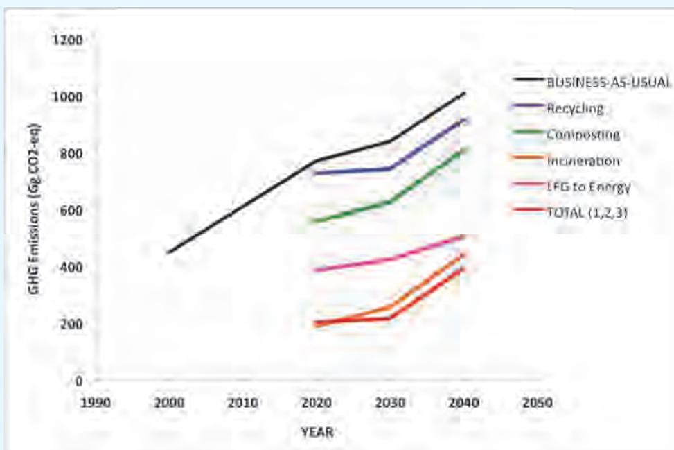
Figure 4.6 - GHG emissions under BAU and selected mitigation options in Solid Waste sector
