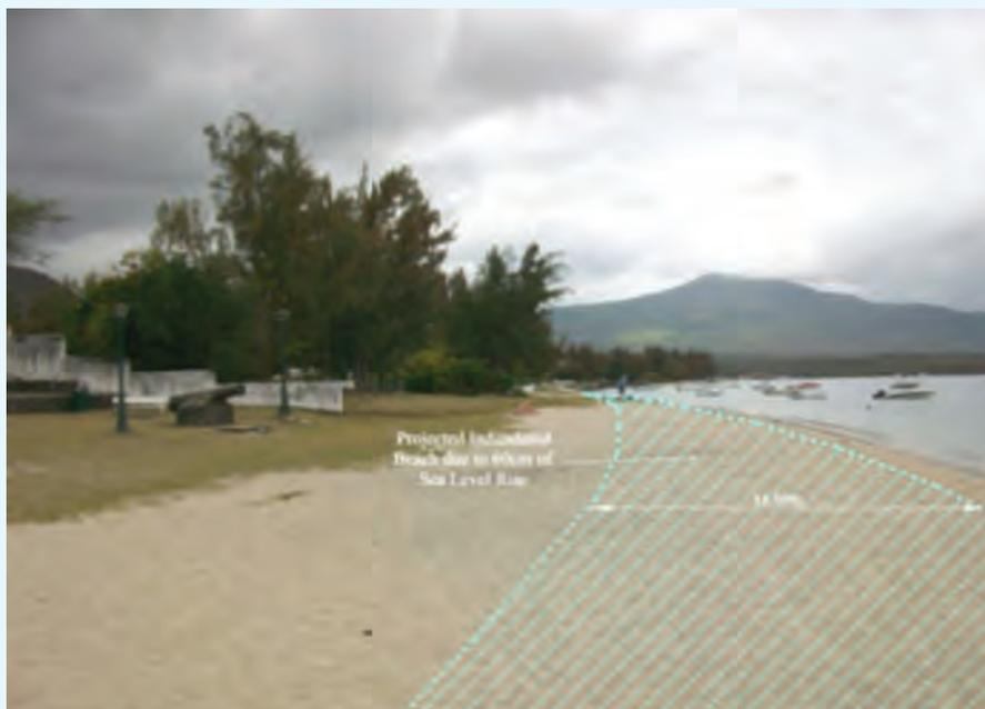
Figure 5.5 - Likely inundation of beach from high water mark at La Preneuse
