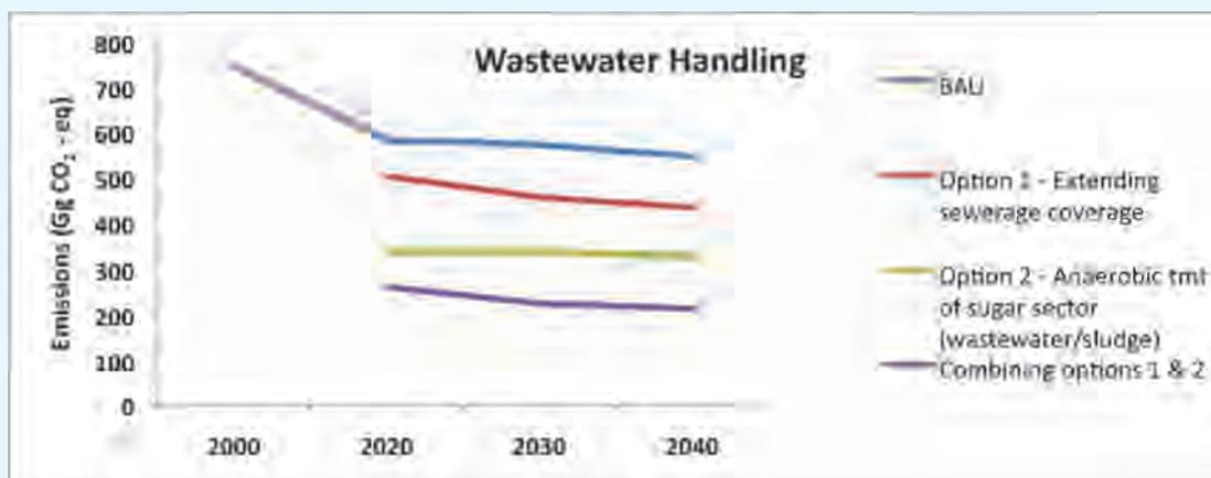
Figure 4.7 - Projected GHG emissions (Gg CO<sub>2</sub>-eq) from mitigation options in Wastewater handling (The Options in the legend refer to those in Table 4.13)
