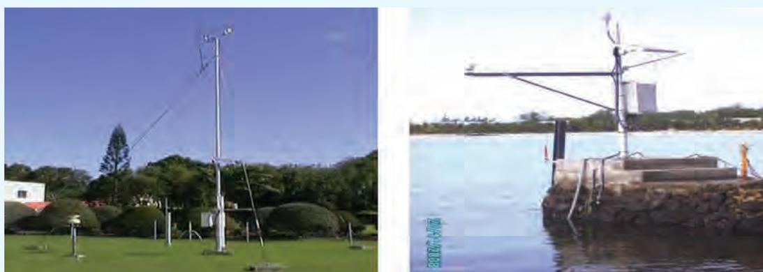
Figure 6.4 - An automatic weather station and, a tide gauge (right). (Courtesy : MMS)
